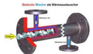
Heat exchanger with spiral mixing elements for high viscosity Media
